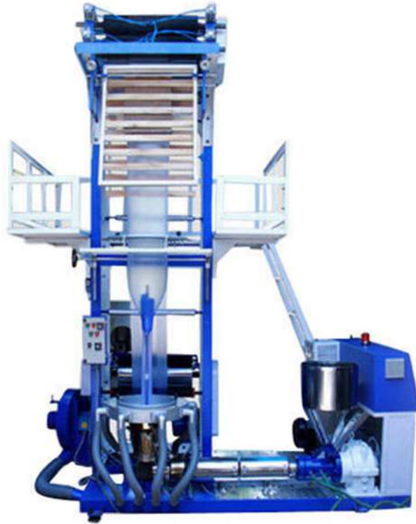
Fig.: Plastic bag extrusion with blown film.
