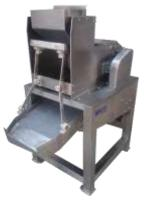
**3. Peanut Grinder:** This machine is designed for grinding oily peanuts into peanut butter or low oil peanuts into peanut powder.
